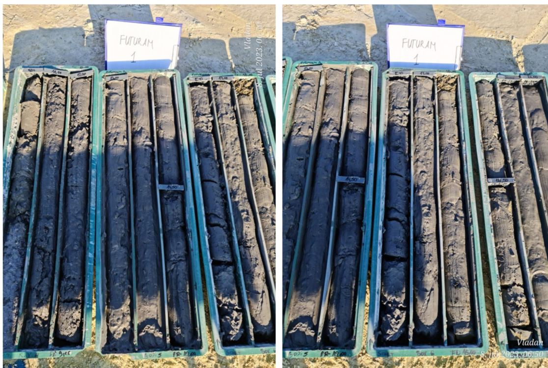
Figure 16: Drilled cores lined up in boxes.
